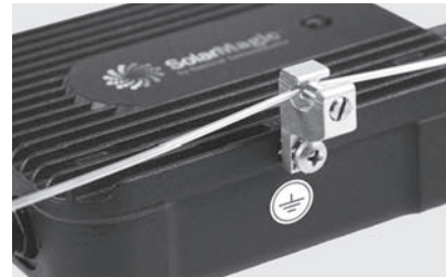
Figure 8. UL-Listed Wet Location Ground Lug with Bare Copper Ground Wire
